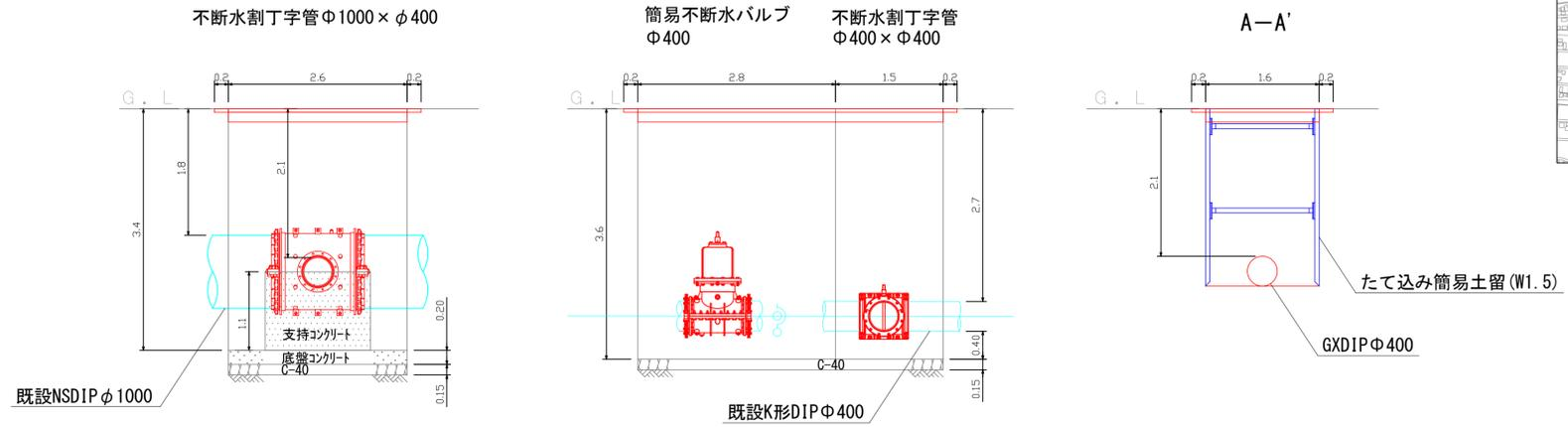
①配水管布設替工事 GXDIPφ400 L=26m (26.0m)
