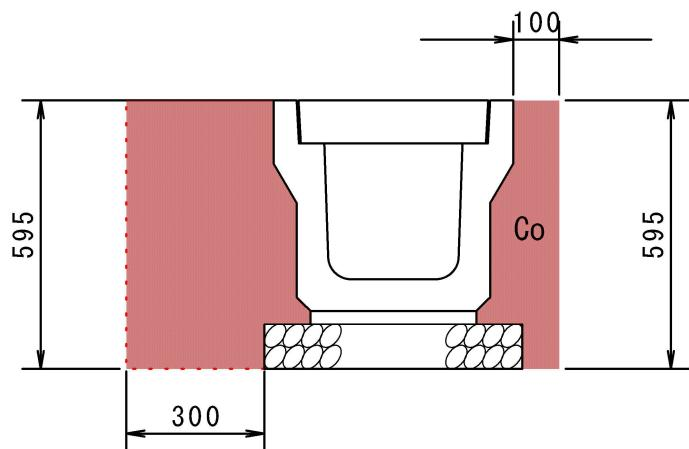
$$\begin{array}{ll} \text{床掘} & A=0.243 \text{ m}^2 \\ \text{埋戻} & A=0.205 \text{ m}^2 \\ \text{埋戻Co} & A=0.074 \text{ m}^2 \end{array}$$
