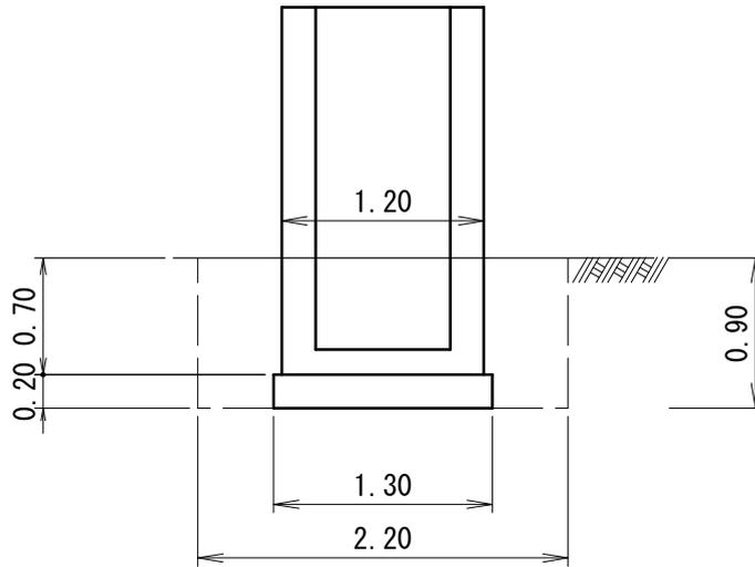
床掘  $V=2.20 \times 2.20 \times 0.90=4.4\text{m}^3$
